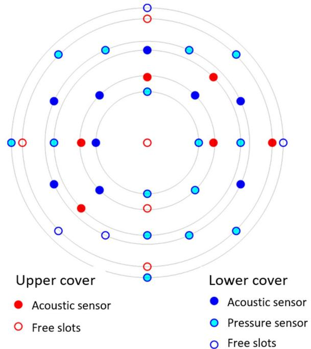
**Fig. 3.** Layout of pressure sensors and acoustic emission sensors in a top view of the setup.
