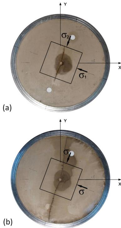
**Fig. 9.** Photo of the sample: (a) hydraulic fracture after injection at a constant flow rate; (b) fracture after injection with a cyclic change in injection pressure.
