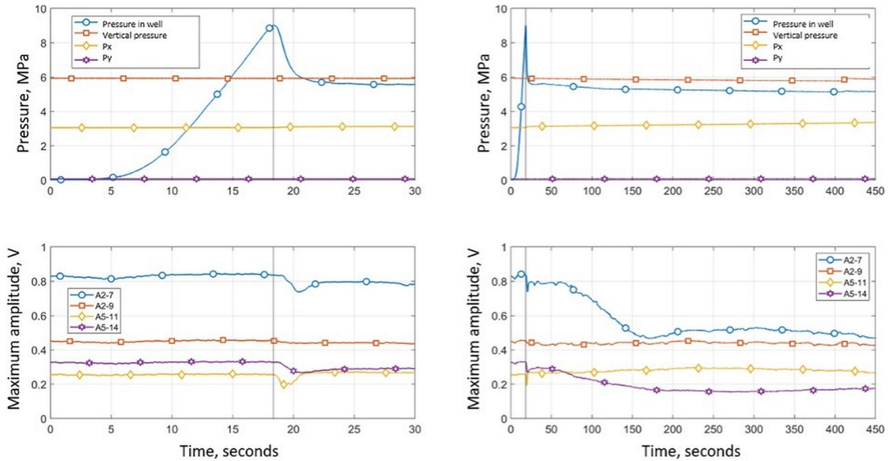
Fig. 7. Initial section (on the left) and complete records (on the right) of the dependences of pressure in the central well and loading pressure on time (upper graphs) and the amplitude of ultrasonic pulses for different receivers (lower graphs).
