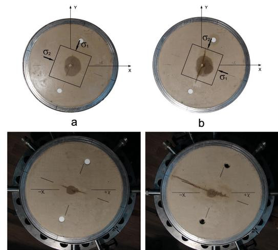
**Fig. 5.** Experiments to determine the effect of changing the orientation of the principal stress axes on the development of hydraulic fractures.
