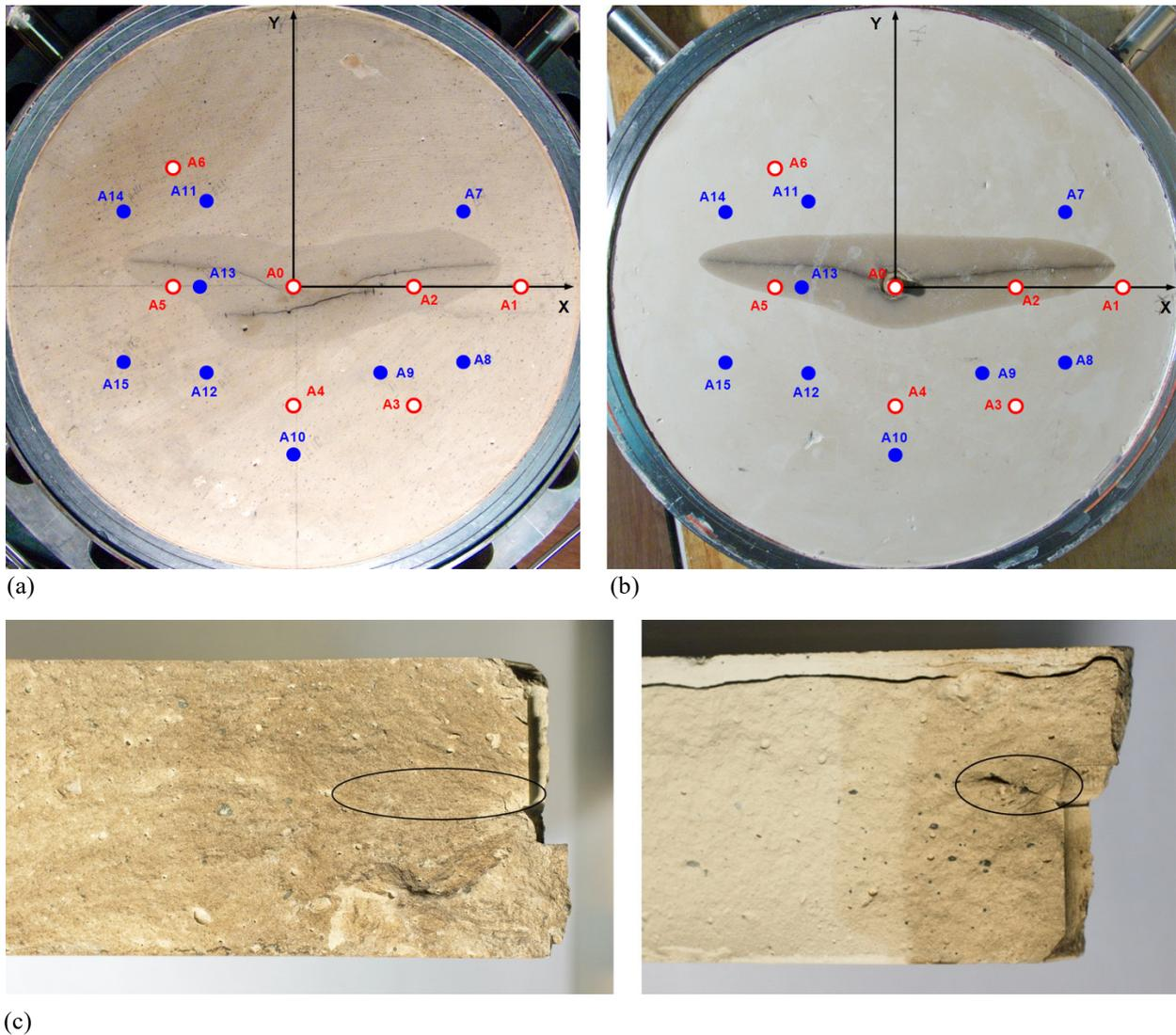
**Fig. 6.** Photographs of the upper (a) and lower (b) surfaces and the sections of the sample (c) after obtaining a secondary hydraulic fracture.
