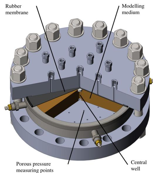
Fig. 1. Diagram of the hydraulic fracturing simulation setup.
